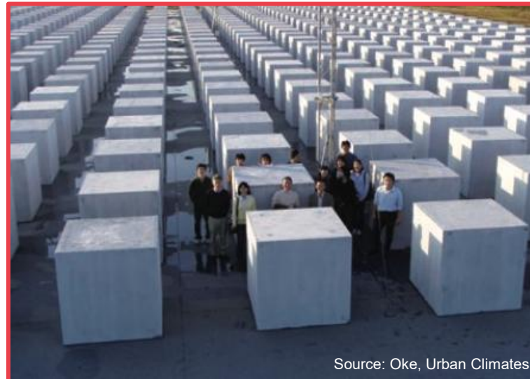
Example of Outdoor Model used for studying effect of urban structure on airflow, turbulence, dispersion, radiation
